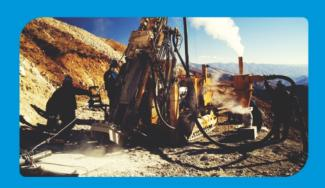
APC owns 4 reverse circulation exploratory rigs and this facilitates drilling up-to 200m.
